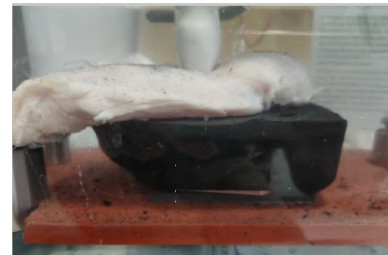
Fig. 3. Experimental setup for homogeneous phantom measurement through aberrating layers. The phantoms were immersed in a water bath during measurement to avoid specular reflections at air inclusions.
